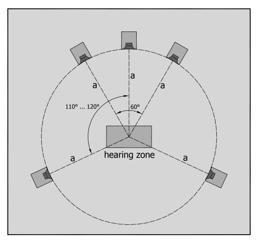
■ Distance between speakers and your listening position  $a = 2 \text{ m} \dots 5 \text{ m} (6'7'' \dots 16'5'')$ In case installation in the prescribed way is not possible in your listening room most decoding
